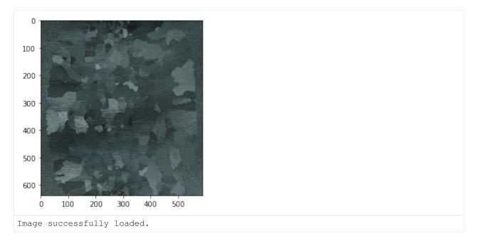
After the image has been loaded and stored in the GS object, we want to remove the noise. Since the interfaces among the grains are important for us, we use median filtering for smoothing as it preserves the contours. The smoothing is governed by the *window size*. The larger this number, the smoother the processed image is, and the higher the computational cost becomes.
