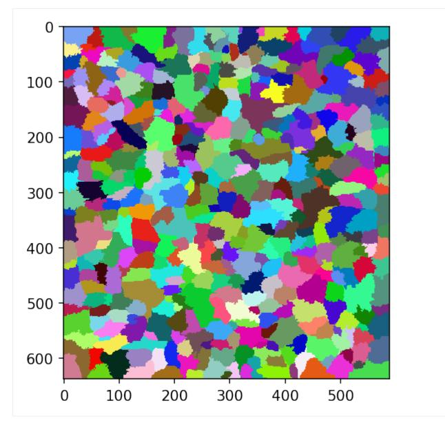
As the superpixel segmentation in the previous step resulted in an oversegmented image, the region adjacency graph is constructed and used to merge some of the neighbouring superpixels based on their similarity with respect to mean colour. Regions connected by edges with smaller weights than a prescribed threshold are combined. As you can see, the number of supersegments decreases.
