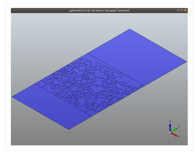
Once we have the spline surfaces, we write them to a STEP file. This allows us to edit the geometry in a CAD program and to generate a mesh for the grains.
